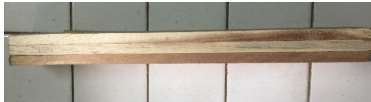
Figure 1 The sample of three-layer homogeneous glulam from jabon wood using tannin adhesive.
