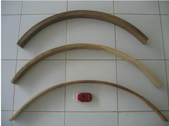
Figure 7. Acacia solid woods with 10 mm, 20 mm, 30 mm thickness that have successfully bent.
