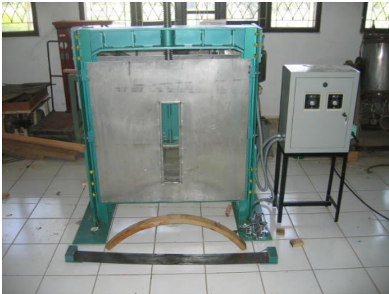
Figure 5. Modified wood bending machine.
