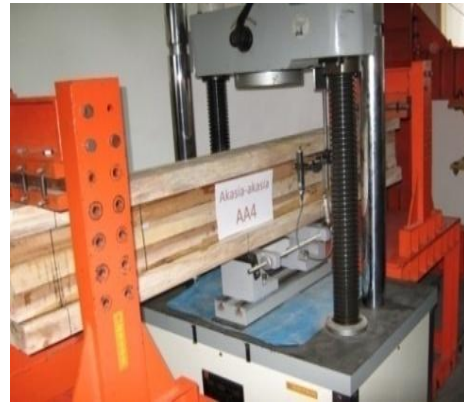
Figure 12 I glulam beam specimens and specimen AA4 under loading test.
