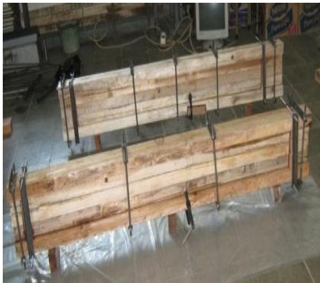
Figure 11 I glulam beam specimens under construction.
