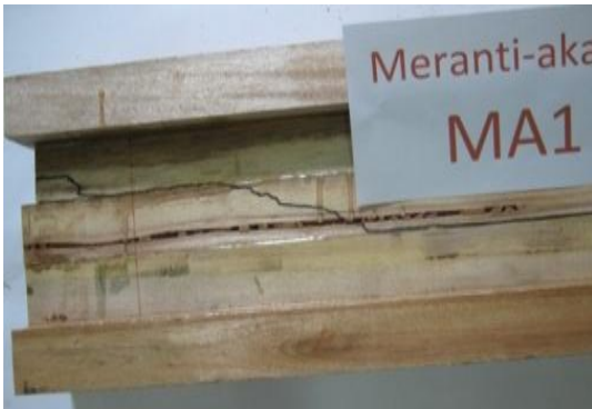
Figure 16 Shear failure modes at web near support of Meranti-Akasia MA1 specimen.
