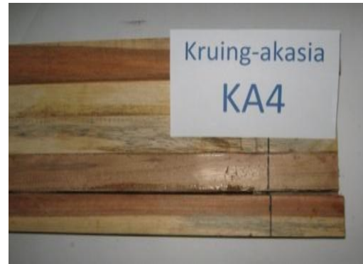
Figure 17 Glue shear failure modes at web-flange surface contact of Keruing-Akasia KA4 specimen.
