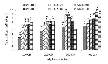
Figure 4 Tear indices of virgin bamboo pulp and OCC pulp mixture at various pulp composition and freeness degree.
