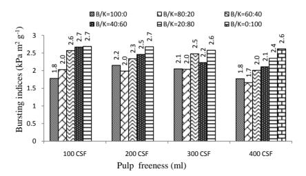
Figure 3 Bursting indices of virgin bamboo and OCC pulp mixture at various compositions and freeness level of pulp.
