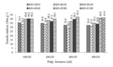
Figure 2 Tensile indices of virgin bamboo and OCC pulp mixture at various composition and freeness of pulp.
