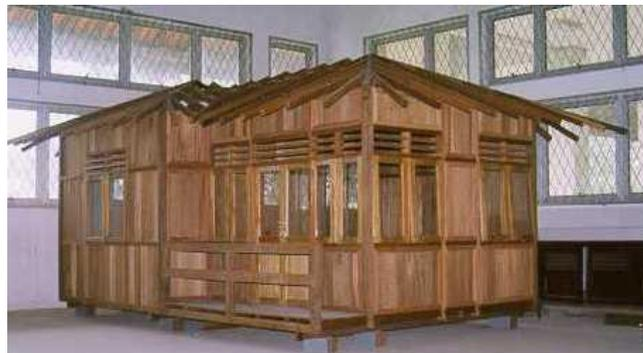
Figure 10. Model of knock down house of 1 : 2 scale located in construction laboratory.
