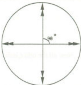
DFT coefficient vector formation for K = 2, 6 . Two rotations of a 4-point DFT coefficient vector geometric formation.
