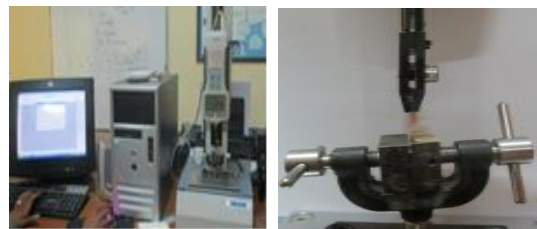
Figure 2: IM ADA Biomechanical Testing Machine Parameters That Were Measured In Biomechanical Testing Are Tensile Load (N) and Tensile Strength (N/mm 2 )
