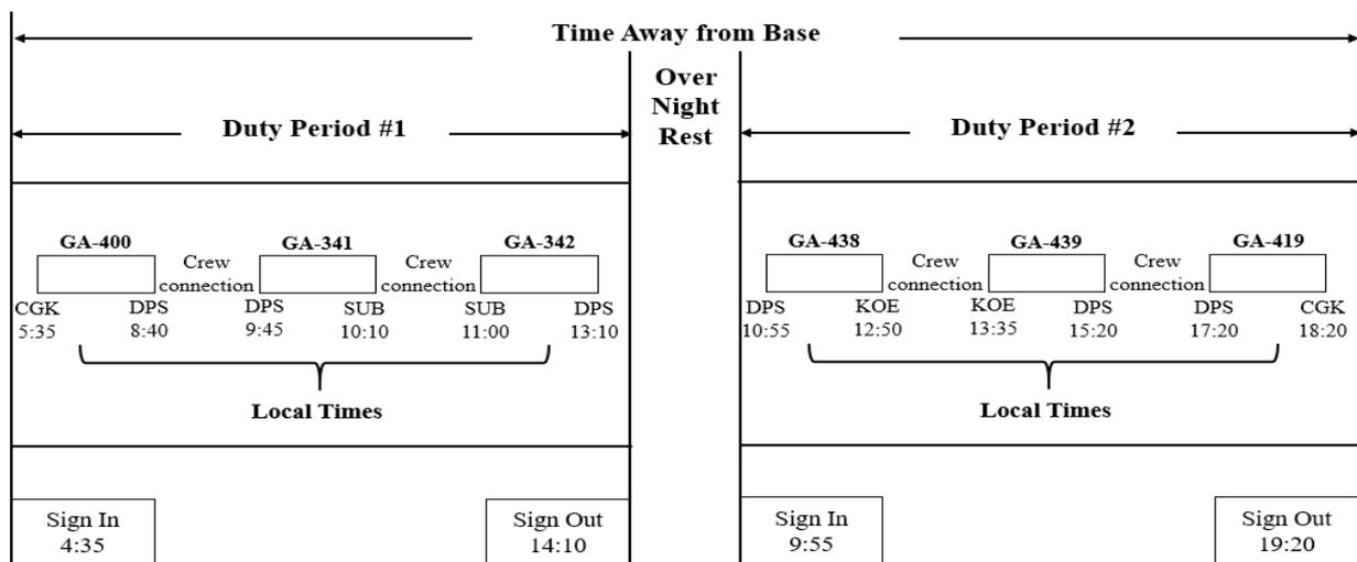
**Figure 1.** A Typical Pairing with Duty Periods, Crew Connection within Duty Periods, Overnight Rests, and Sign-In and Sign-Out Times. Adopted from Bazargan [3]
