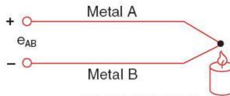
■ Gambar 5. Prinsip Kerja Thermocouple [6]
