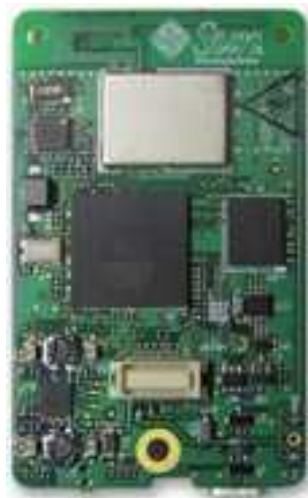
■ Gambar 19. Sirkit node sensor
