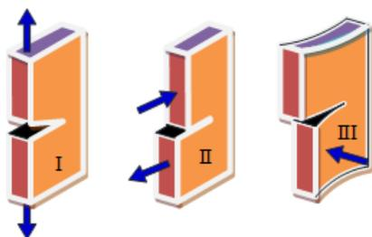
Figure 1 Types of loading. (I) opening Mode, (II) Sliding Mode, (III) Tearing mode [8]
