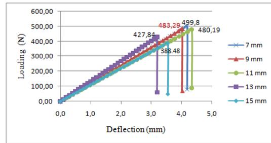
Figure 6. Graph of test result on fiber orientation 0/90°
