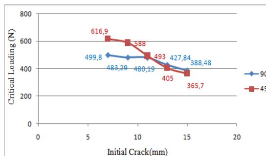
Figure 8. Graph of orientation of fiber 0/90° with fiber orientation 0/45°
