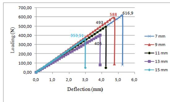
Figure 7. Graph of test results at 0/45° fiber orientation
