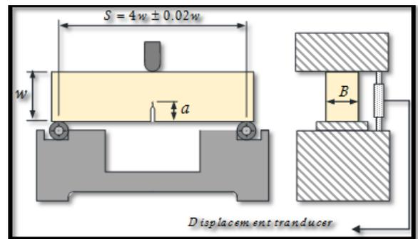
Figure 4. Crack testing standards ASTM D5045
