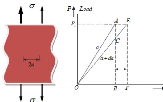
Figure 2. Griffith energy criterion for fixed grip (a) Crack with fixed tip, (b) Elastic energy [10]
