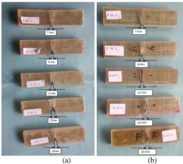
Figure 11. Fracture propagation at (a) orientation  $0/45^\circ$  and (b) orientation  $0/90^\circ$
