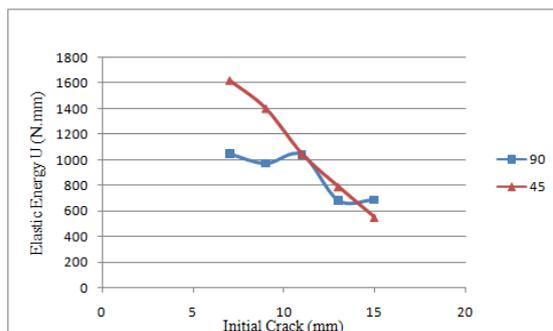
Figure 9. Elastic energy vs initial crack
