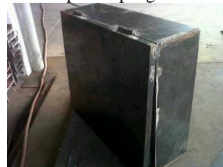
Gambar 9 Box panel hasil proses welding
