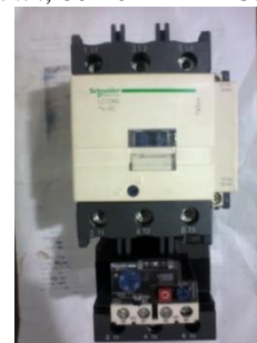
Gambar 22 Magnetic Contactor dan Overload Relay
