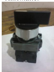
Gambar 16 Main Auto Selector Switch
