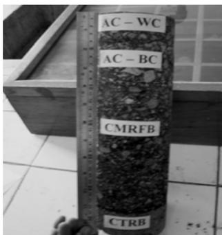
**Gambar 11.** Contoh hasil *Core drill*
