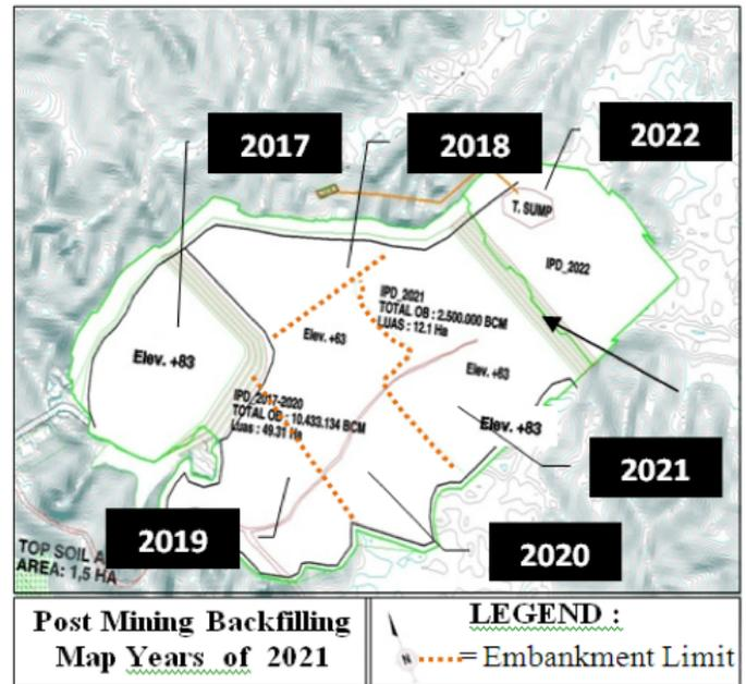
**Figure 6.** Design embankment (year 2021) backfilling year-1st
