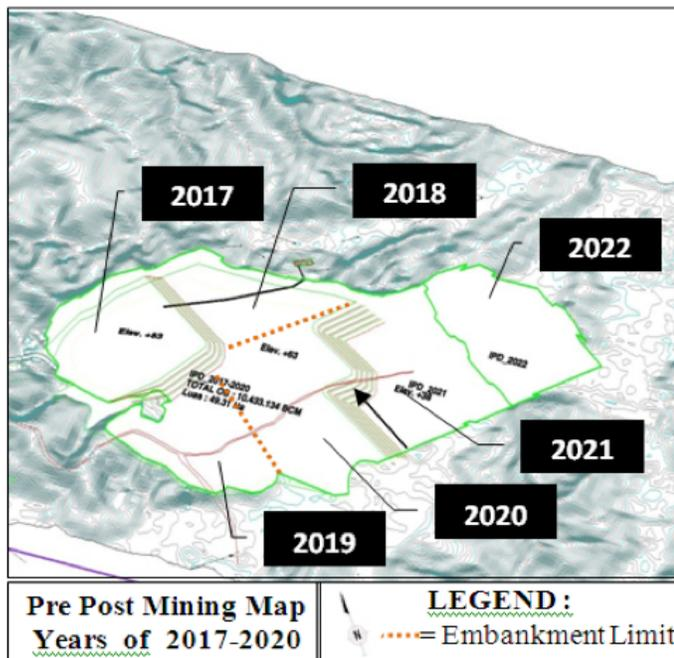
**Figure 5.** Design embankment (2017-2020) pre-post mining
