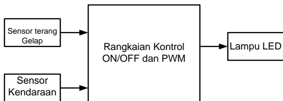
Gambar 8. Blok diagram kontrol lampu PDU
