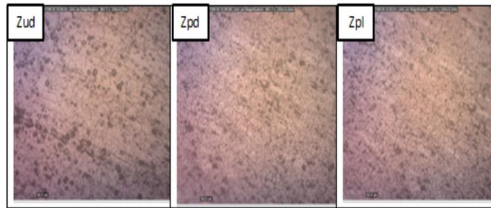
Fig. 7. Microstructure of Zud, Zpd (HAZ) and Zpl zones of the specimen rotated at 4000 rpm and 8 MPa for 80 S
