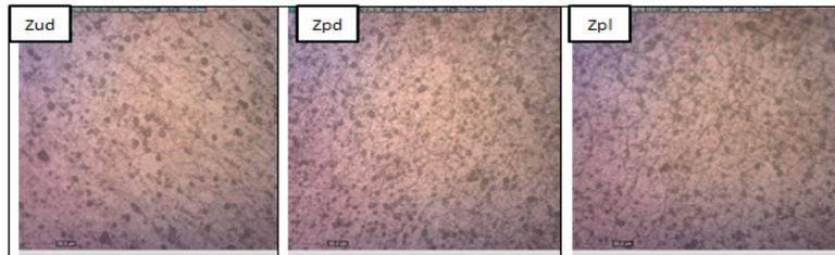
Fig. 4. Microstructure of Zud, Zpd (HAZ) and Zpl zones of the specimen rotated at 2850 rpm and 8 MPa for 60 S
