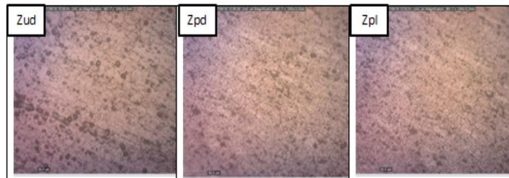
Fig. 6. Microstructure of Zud, Zpd (HAZ) and Zpl zones of the specimen rotated at 4000 rpm and 8 MPa for 60 S
