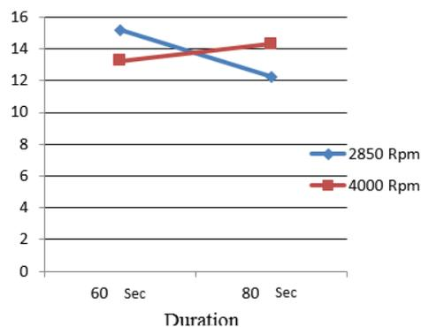
Fig. 2. Average Tensile Strength Resulted from Friction Welding
