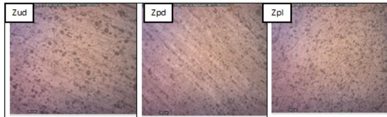
Fig. 5. Microstructure of Zud, Zpd (HAZ) and Zpl zones of the specimen rotated at 2850 rpm and 8 MPa for 80 S
