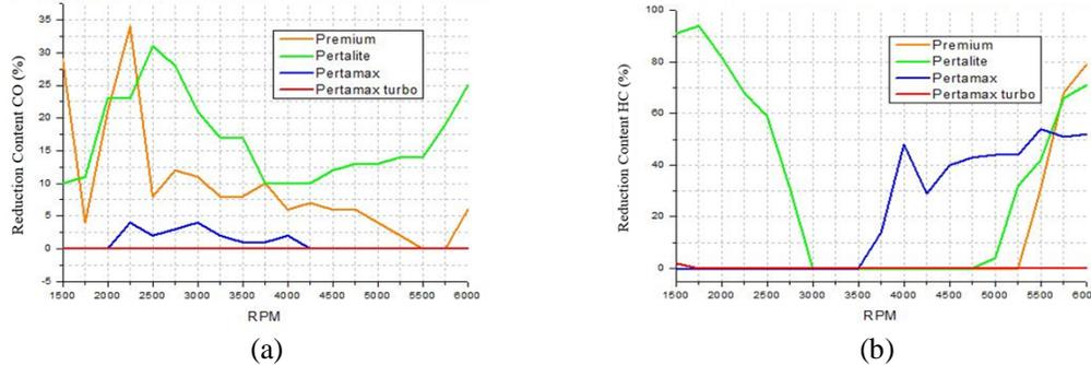
Fig. 6. Percentage of emission reduction per fuel (a) CO (b) HC content
