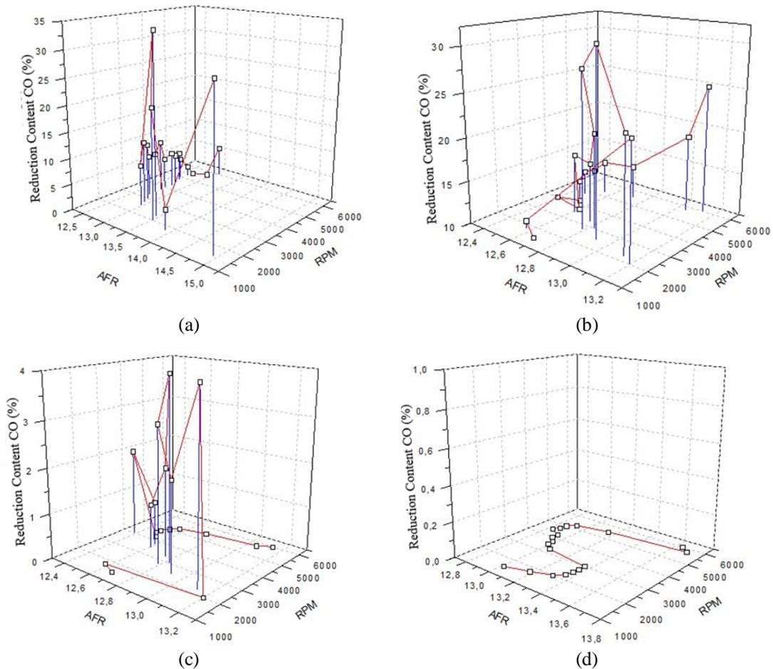
Fig. 8. Effect of AFR on decrease of CO content of each fuel (a) Premium (b) Peralite (c) Pertamina (d) Pertamina turbo
