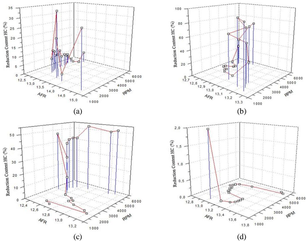
Fig. 9. Effect of AFR on decreasing of HC content of each fuel (a) Premium (b) Peralite (c) Pertamina (d) Pertamina turbo
