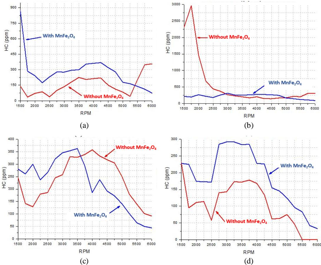
Fig. 4. Comparison graph of HC content without MnFe<sub>2</sub>O<sub>4</sub> and with MnFe<sub>2</sub>O<sub>4</sub> per fuel (a) Premium (b) Peralite (c) Pertamina (d) Pertamina turbo
