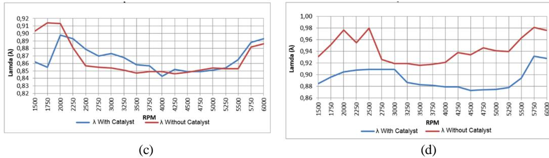
Fig. 3. Comparison graph of lamda ( $\lambda$ ) without  $MnFe_2O_4$  and with  $MnFe_2O_4$  per fuel (a) Premium (b) Peralite (c) Pertamax (d) Pertamax turbo
