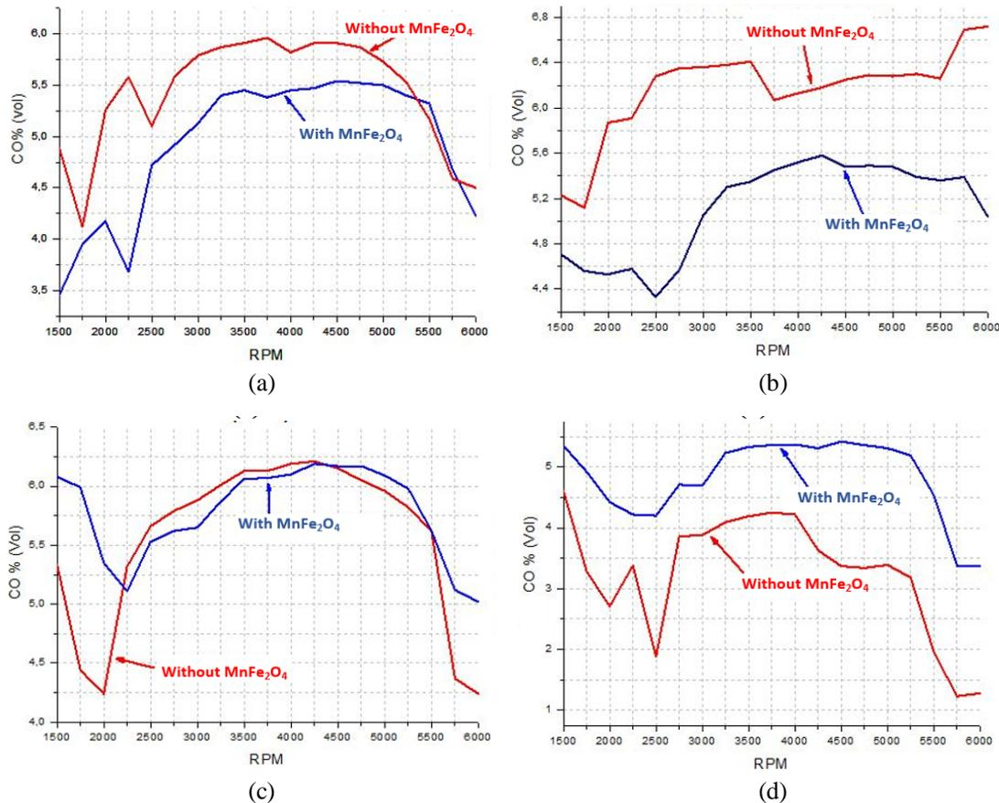
Fig. 2. Comparison graph of CO content without  $MnFe_2O_4$  and with  $MnFe_2O_4$  per fuel (a) Premium (b) Pertalite (c) Pertamina (d) Pertamina turbo
