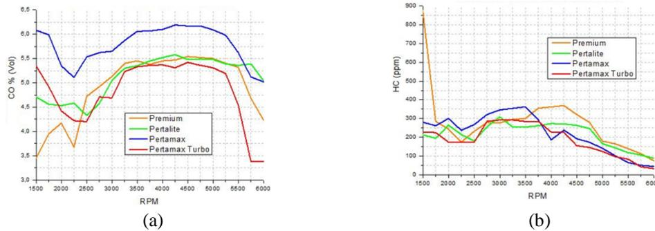
Fig. 7. Emissions levels per fuel (a) CO (b) HC content
