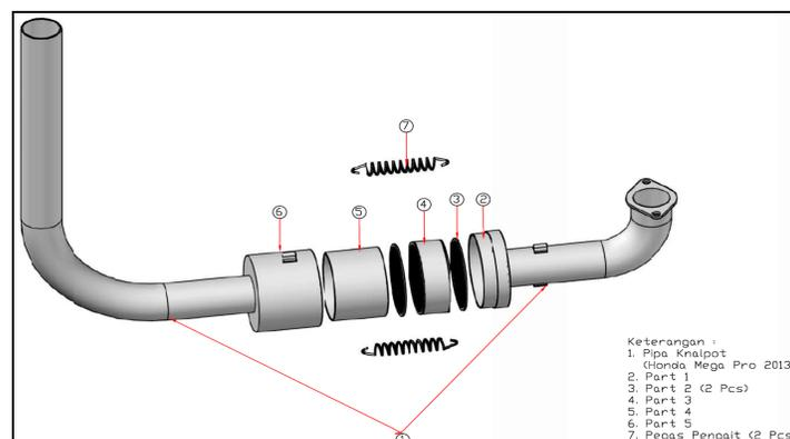
Fig. 1. Design of reactor tubes
