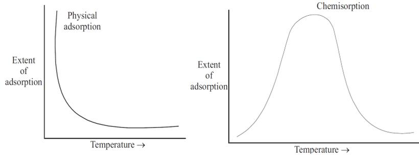
Fig. 5. Effects of temperature on (a) Physical adsorption (b) Chemisorption
