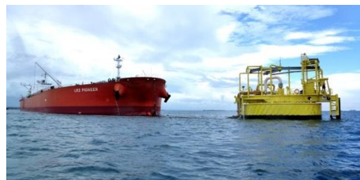
Figure 1. Single buoy mooring system [5]
