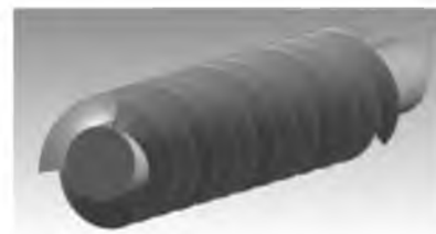
Gambar 2. sudu turbin archimedes screw (5)
