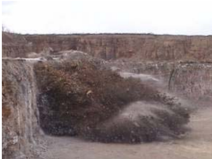
Figure 3. Blast process in a mine produces fragmented rocks and a series of blast-generated vibrations ( www.terradinamica.com/program.htm ).
