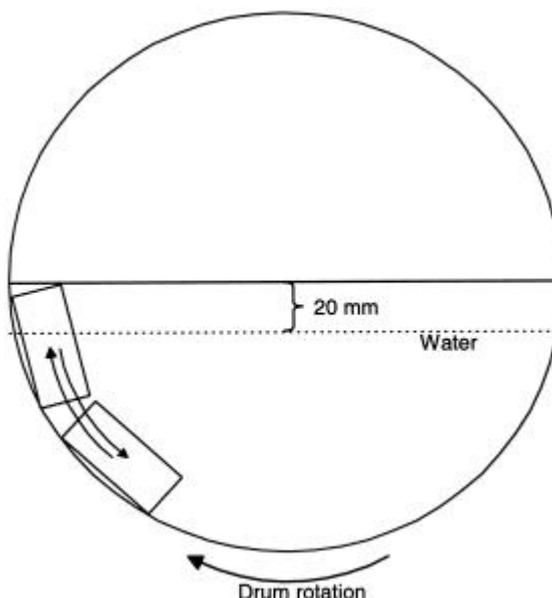
Figure 5. Rectangular specimens in the slake-durability drum.
