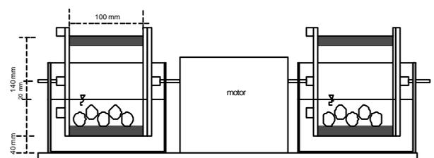
Figure 1. The slake-durability test apparatus.
