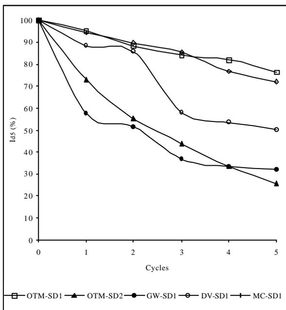
Figure 2. Five-cycle slake-durability tests.
