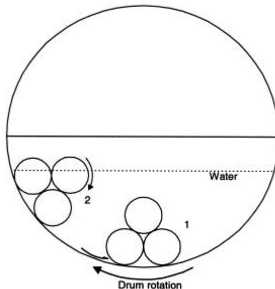
Figure 4. Rounded rock specimen in the slake-durability drum.
