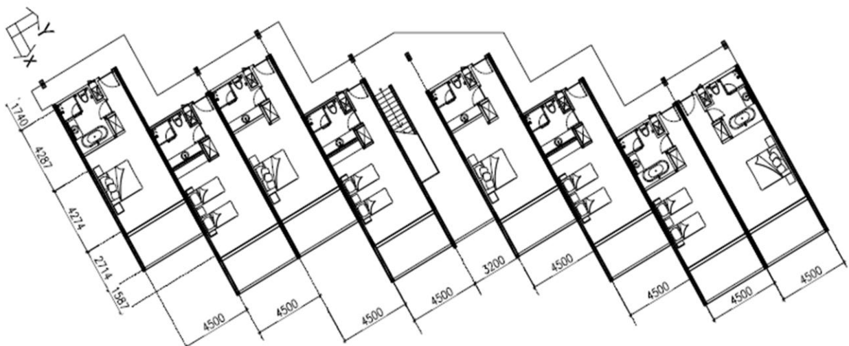
Figure 1. Architectural Plan of 1 st – 4 th Floor with Thick Walls between Rooms
