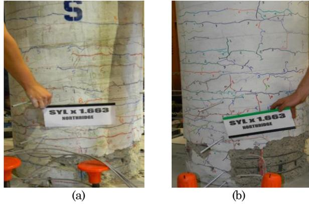
Figure 11. Spalling on South Face of North Column (a) With and (b) Without Live Load after 350% DE Run
