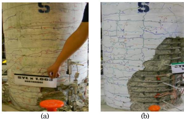
Figure 10. Spalling on South Face of South Column (a) With and (b) Without Live Load after 350% DE Run
