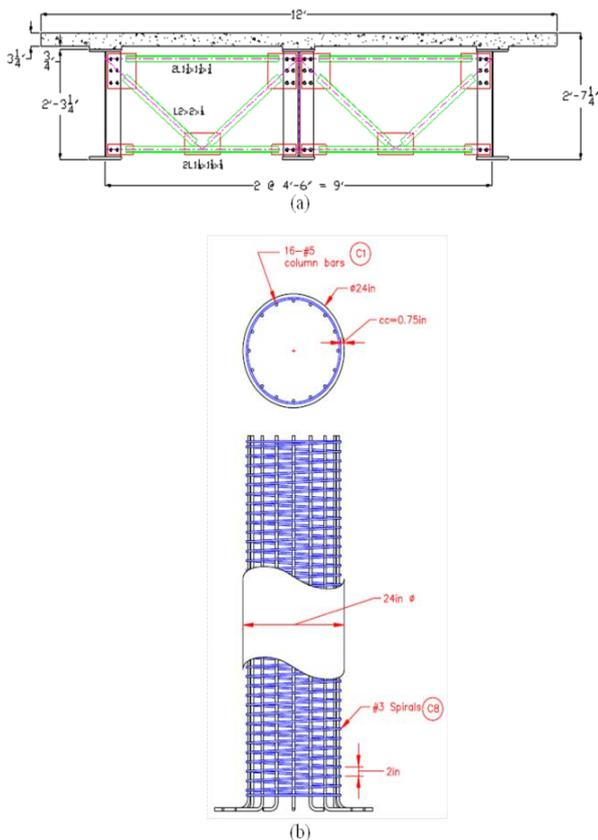
Figure 3. Typical Superstructure and Column Details
