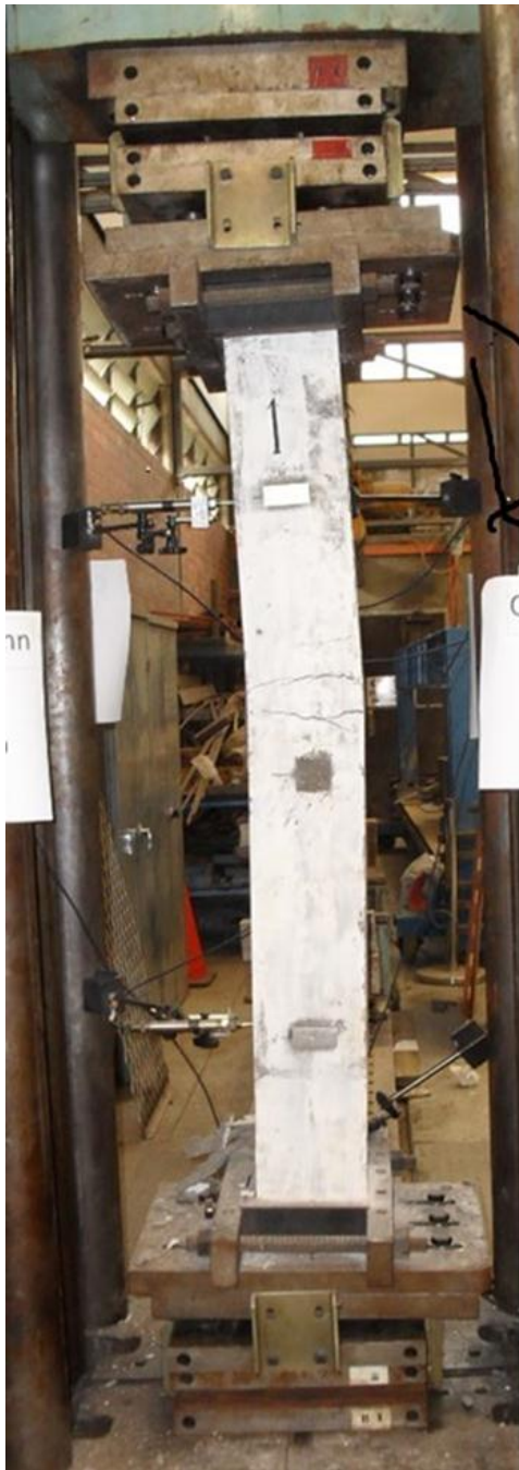
Figure 9. Test of Geopolymer Concrete Column in Combined Axial Compression and Biaxial Bending
