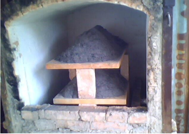
Figure 2. Bamboo Leaf Ash after Calcinations in Furnace
