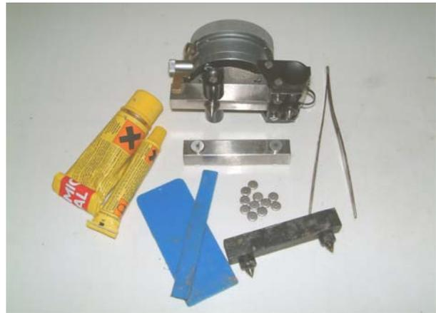
Figure 2. The 50 mm Demec gauge set.
