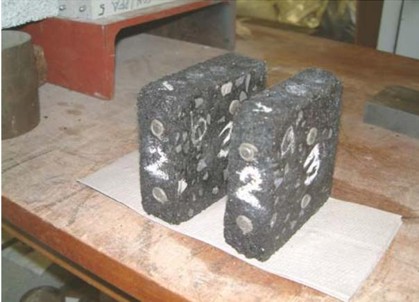
Figure 1. The samples for the moisture adsorption (MA) test.
