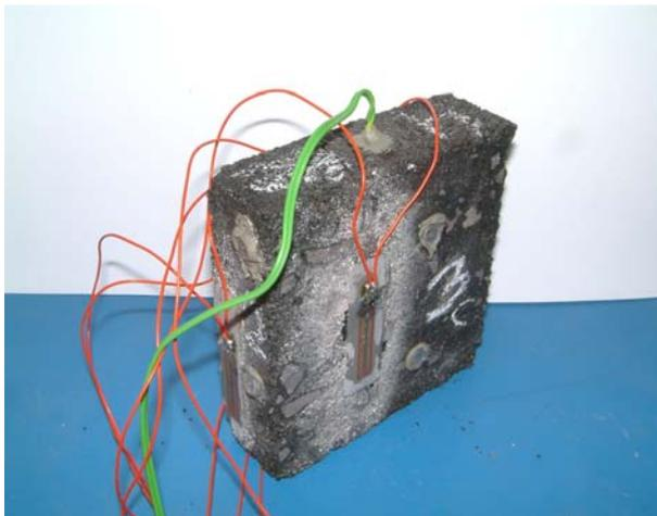
**Figure 4.** Preparation of sample completed with ers gauges and a thermocouple.
