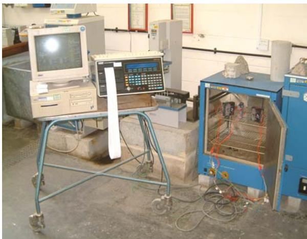
**Figure 5.** Strain measurement by means of ers gauge recorded by a data logger and computer.
