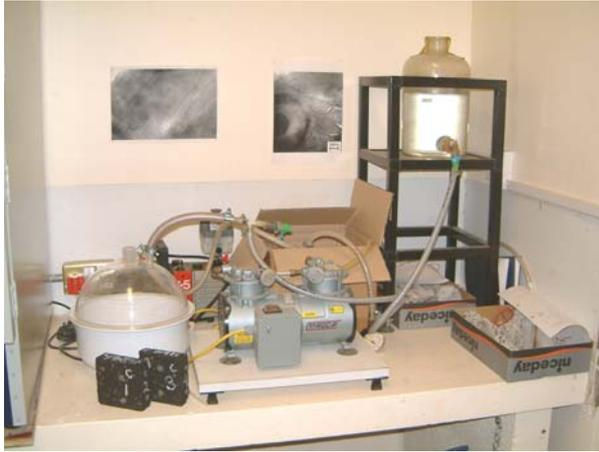
Figure 10. The vacuum saturation equipment.
