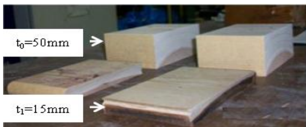
Figure 1. Typical Thickness of Softwood and Compressed Wood before and after the Compressing Process [5].
