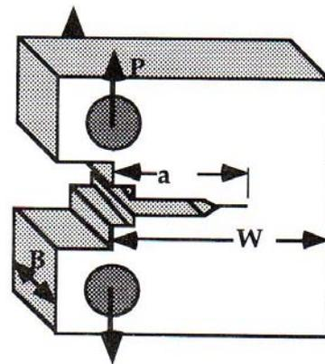
Figure 3. Mode I Fracture Testing Specimen Geometry (CT-Specimen) [7]
