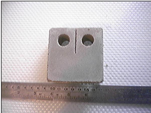
Figure 10. Actual Size of the Mode I Fracture Testing of CT-Specimen
