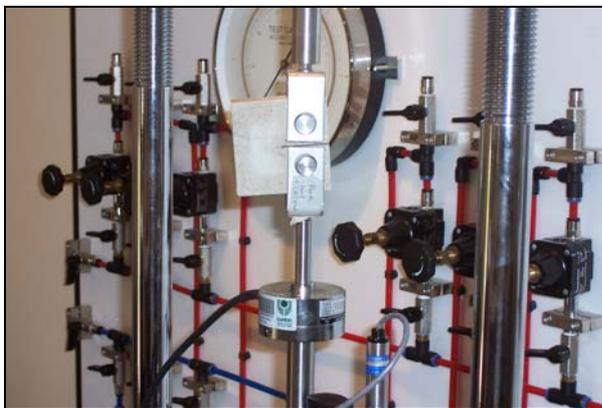
Figure 11. Set up of Mode I Fracture Testing of CT-Specimen
