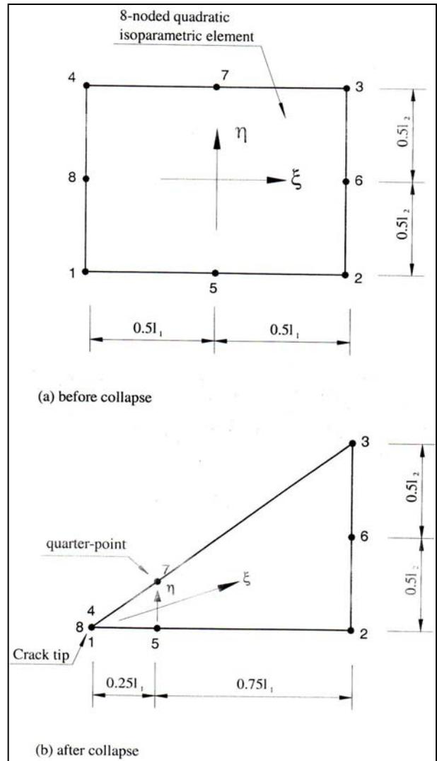
Figure 5. Formation of Triangular Crack-Tip Element From 8-Noded Quadratic Quadrilateral Element
