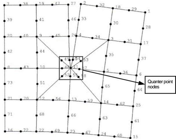
Figure 7. Illustration of Quarter Point Nodes in Finite Element Mesh
