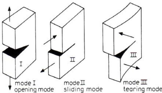
Figure 1. Typical Modes of Fracture
