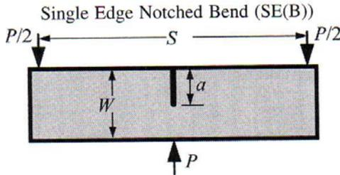
Figure 4. Typical Geometry of Mode I Fracture Testing of Beam Specimen [7]
