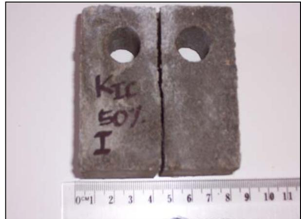
Figure 13. Typical Failure Pattern of Mode I Fracture Testing (CT-Specimen)
