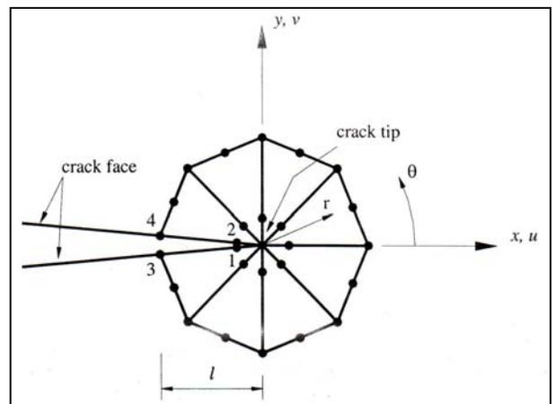
Figure 6. Quarter-Point Elements Modeled Around Crack Tip [8]
