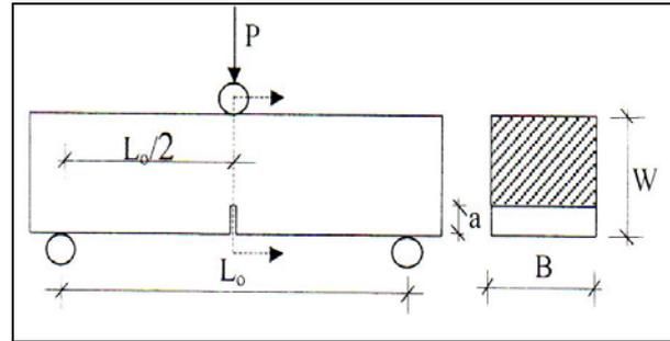
Figure 12. Geometry of Beam Specimen Tested [10]
