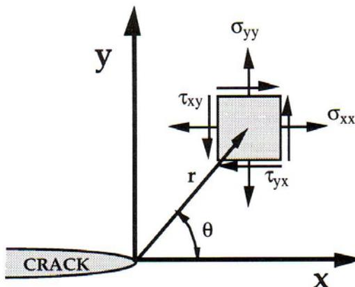
Figure 2. Stresses Near The Tip of a Crack in an Elastic Material
