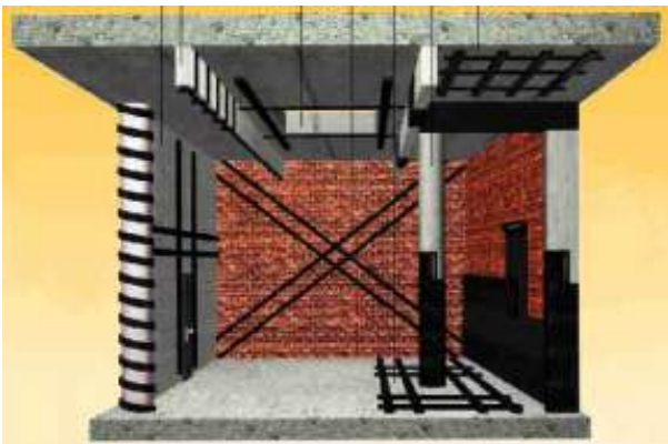
Figure 1. Strengthening for Concrete Structure using FRP System
