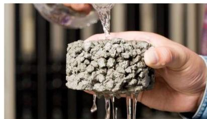
**Gambar 1.** *Pervious Concrete.*
