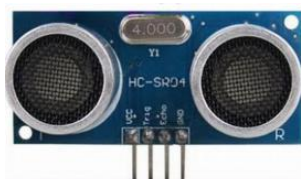
Gambar 4. Modul Sensor Ultrasonik HC-SR04
