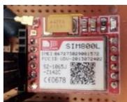
Gambar 6 Modem GSM/GPRS SIM800L
