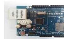
Gambar 3 Ethernet Shield
