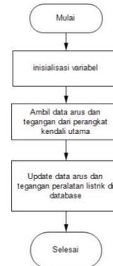
Gambar 14 *Flowchart* *Function* update data peralatan listrik
