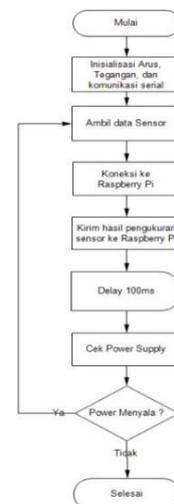
Gambar 11. *Flowchart* Kode Program Arduino
