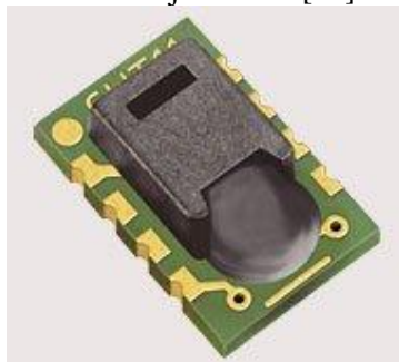
Gambar 4. Sensor SHT-11 (sumber: fahmizal.wordpress.com )
