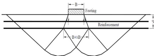
Gambar 1. Mekanisme wide slab
