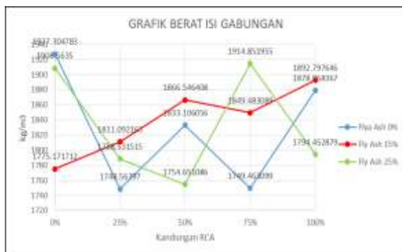
Gambar 6. Grafik berat isi beton porous.
