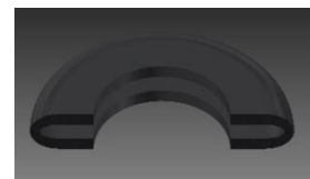
Gambar 4. Penampang melintang gasket
