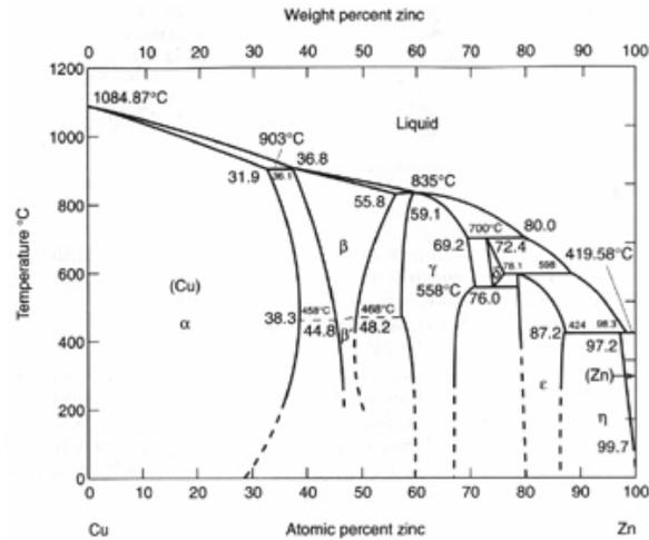
Fig. 3. Diagram of phase brass (Cu-Zn)
