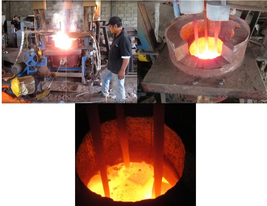
Figure 4. Nickel dimensions of 3 \times 3 \text{ cm}^2 can melt perfectly in EA Furnace
