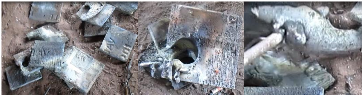
Figure 3. Nickel Dimension of 15 x 15 cm 2 can't melt perfectly in EA Furnace
