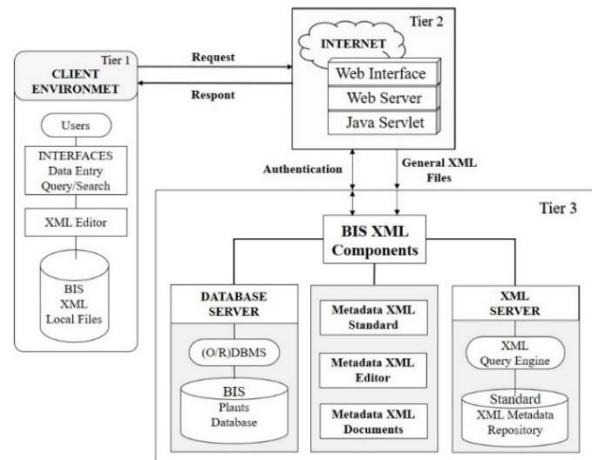
Fig. 2. Figure 3: Three-tier architecture for biodiversity information system
