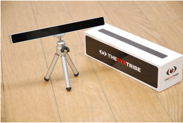
Fig. 1. The used eye tracker device called the Eye Tribe (source: www.ippinka.com).
