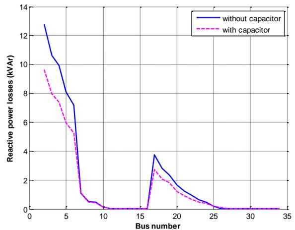
Fig. 6. Reactive power line losses of IEEE 34-bus radial distribution system.
