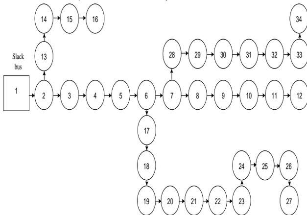
Fig. 3. The schematic diagram of the 34-bus radial distribution system.
