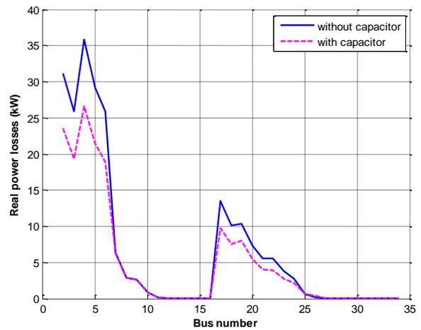
Fig. 5. Real power line losses of IEEE 34-bus radial distribution system.
