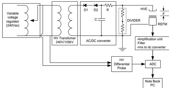
Fig. 4. The general of REFM calibration setup
