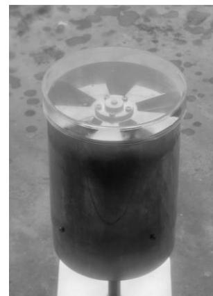
**Fig. 1.** Rotating-vane electric field mill.
