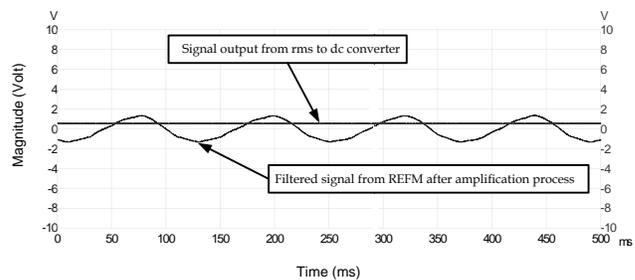
Fig. 3. A sample of signal output from rms to dc converter
