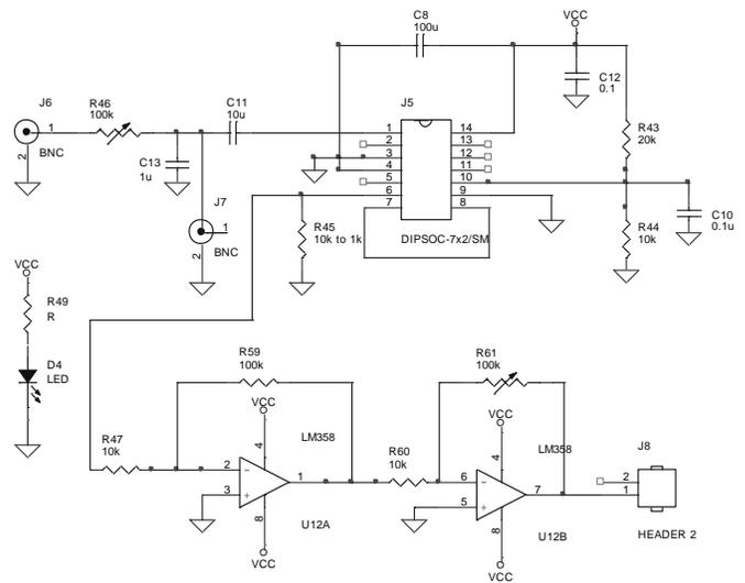
Fig. 2. The filter, converter, and conditioner unit schematic diagram
