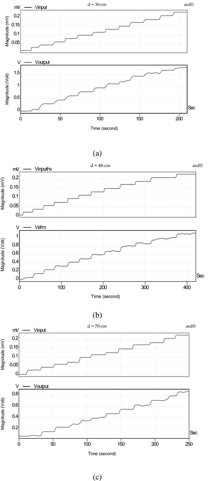
Fig. 5. The results of online calibration measurement according to the distance of the cloud simulation to the REFM, (a) 30-cm, (b) 48-cm, and (c) 70-cm.
