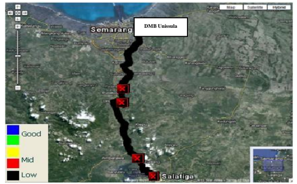
Fig. 5. The Result of the Main road drive test in the Southern Area
