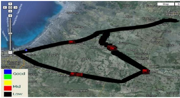
Fig. 4. The Result of the Main road drive test in the east of the Transmitter
