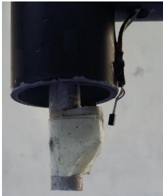
Figure 2. Position of Hall Effect Sensor
