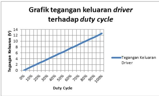
Gambar 4. Grafik Hasil Pengujian Driver Motor (High Current 30A DC Motor Driver)
