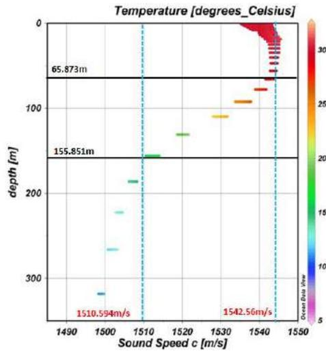
Figure 27. Sound Speed range estimated based on thermocline limit, in July 2014.
