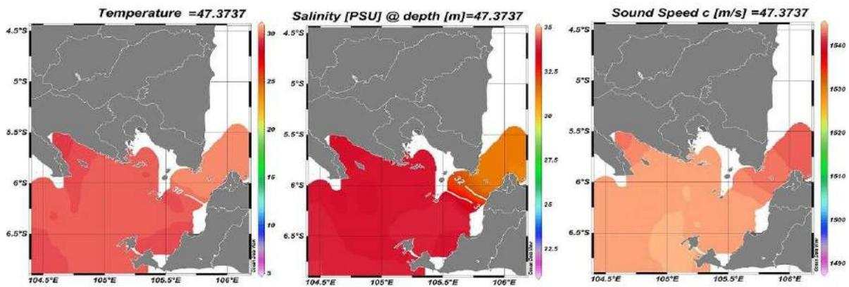
Figure 18. Spatial horizontally distribution of temperature, salinity and sound speed, in July 2014, at 47 m depth.
