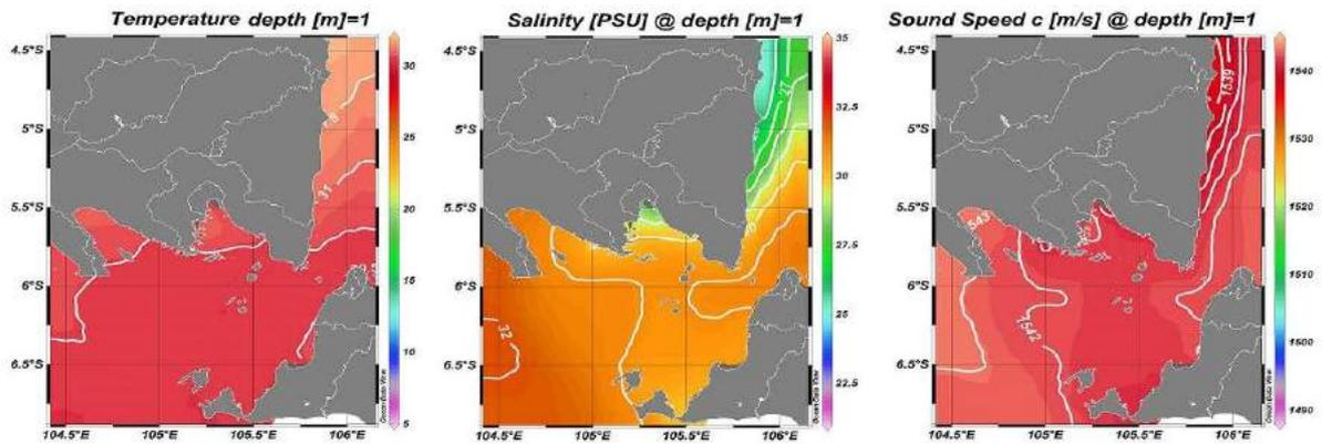
Figure 14. Spatial horizontally distribution of temperature, salinity and sound speed, in April 2014, at 1 m depth.
