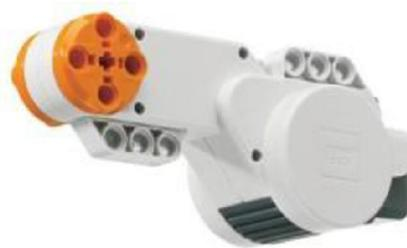
**Gambar 5.** Servo Motor
