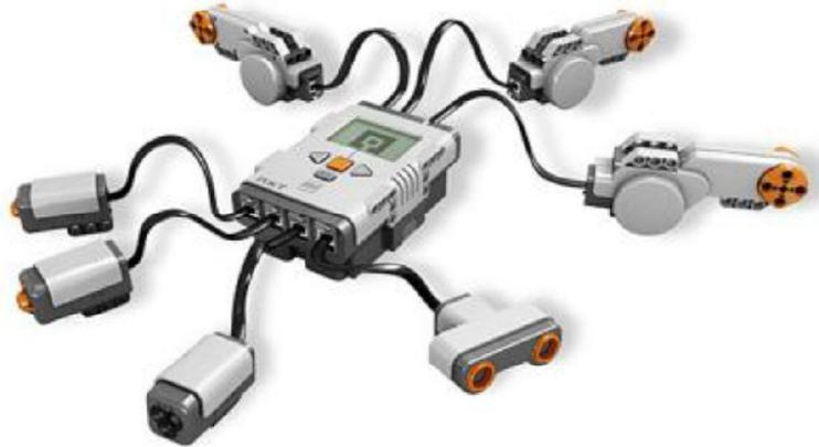
**Gambar 1.** Komponen I/O Lego Mindstorms NXT 2.0
