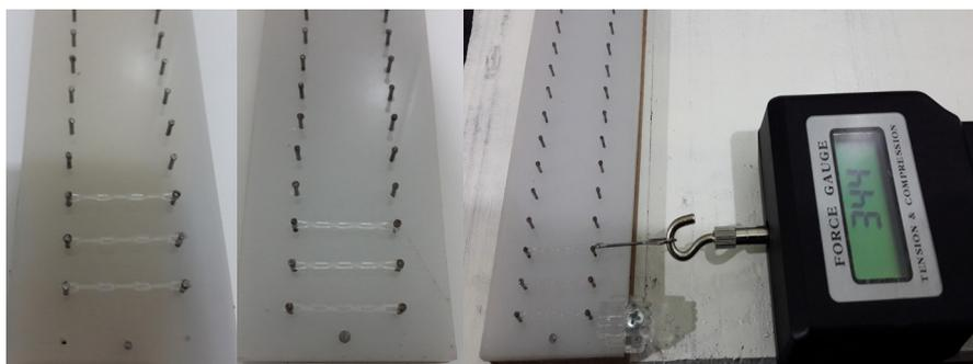
Figure 1. Power chain force measurement with the force gauge
