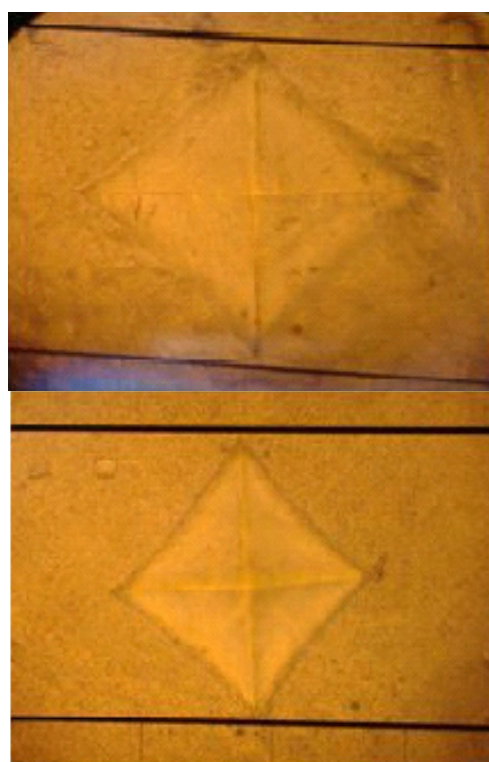
Figure 1. Surface hardness indentation after 2-day soaking Upper: Thermoplastic nylon resin; Lower: Heat-cured acrylic resin.
